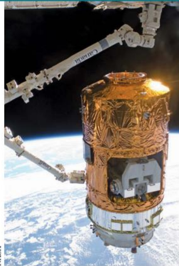
The International Space Station's Canadarm2 grapples the Kounotori2 H-II Transfer Vehicle as it approaches the station in 2011.
